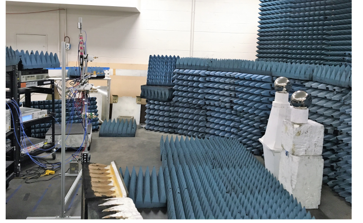
Fig. 7. Photograph of the experimental setup in a semi-enclosed arch range. The targets consisted of one or two metal reflecting targets.
