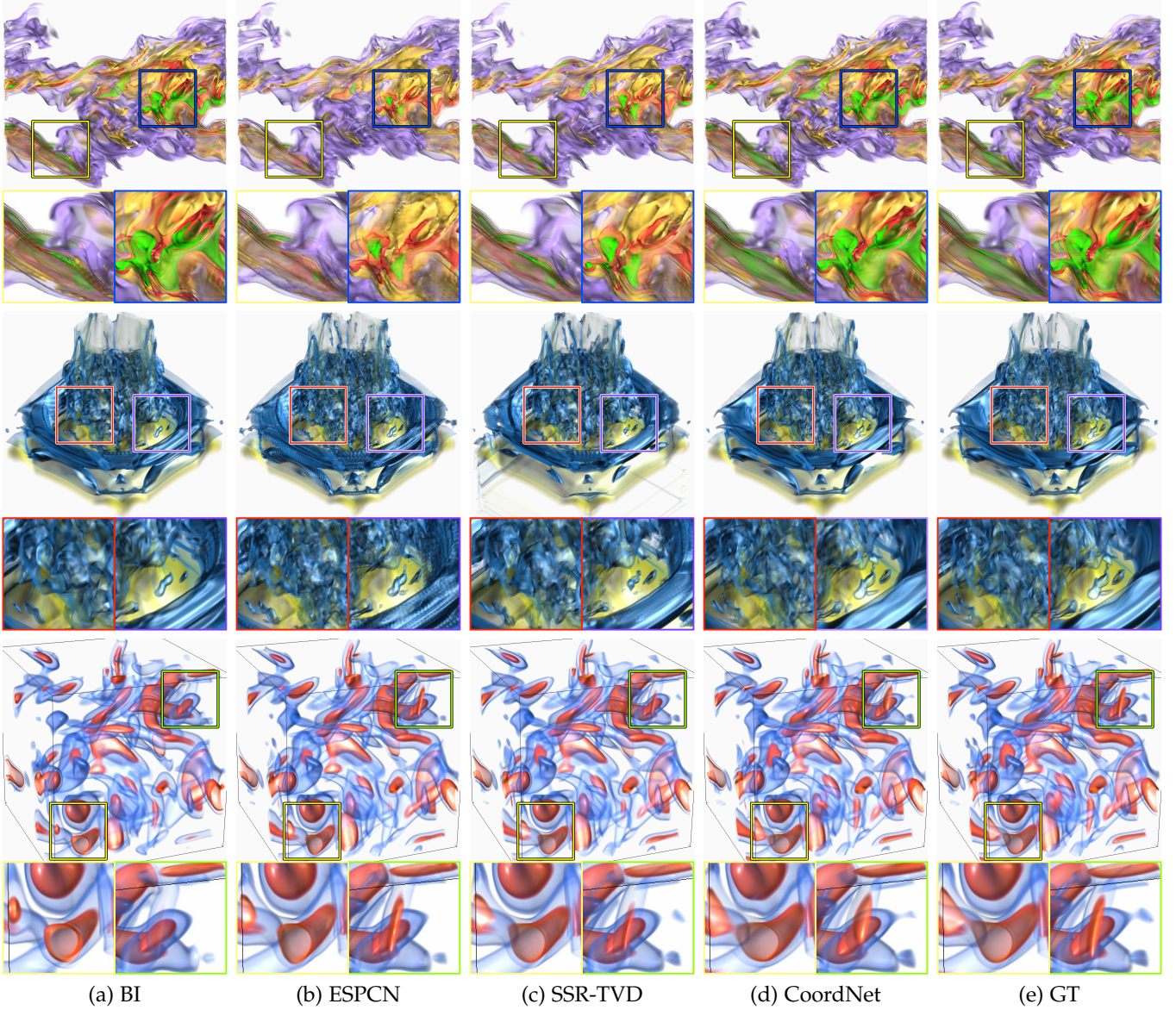
Fig. 9: Volume rendering results for the SSR task with an upscaling factor of 4\times . Top to bottom: combustion (HR), ionization (T), and vortex. The quantitative values are shown in Table 6.
