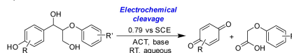
Figure 4. Selective examples of C–O and/or C–C bonds cleavages: (a) C α –C β bond cleavage, (b) C β –O ether bond cleavage, and (c) C aryl –C α bond cleavage. The recently developed redox methods in mild conditions are present in red for photochemical methods and in blue for electrochemical strategies.
