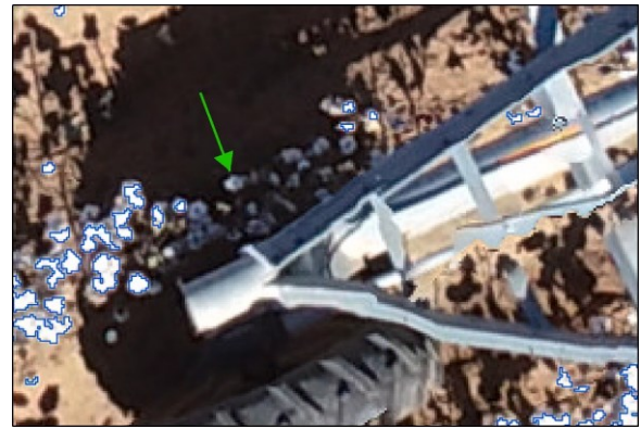
Fig. 7. Omission error resulting from pivot shadowed pixels at experiment site III.
