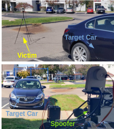
Figure 6: A spoofer launches a malicious frustum attack against a victim AV using a target car. Spoof points are placed at any distance within the frustum behind the target car to obtain false positive, false negative, and/or translation outcomes.
