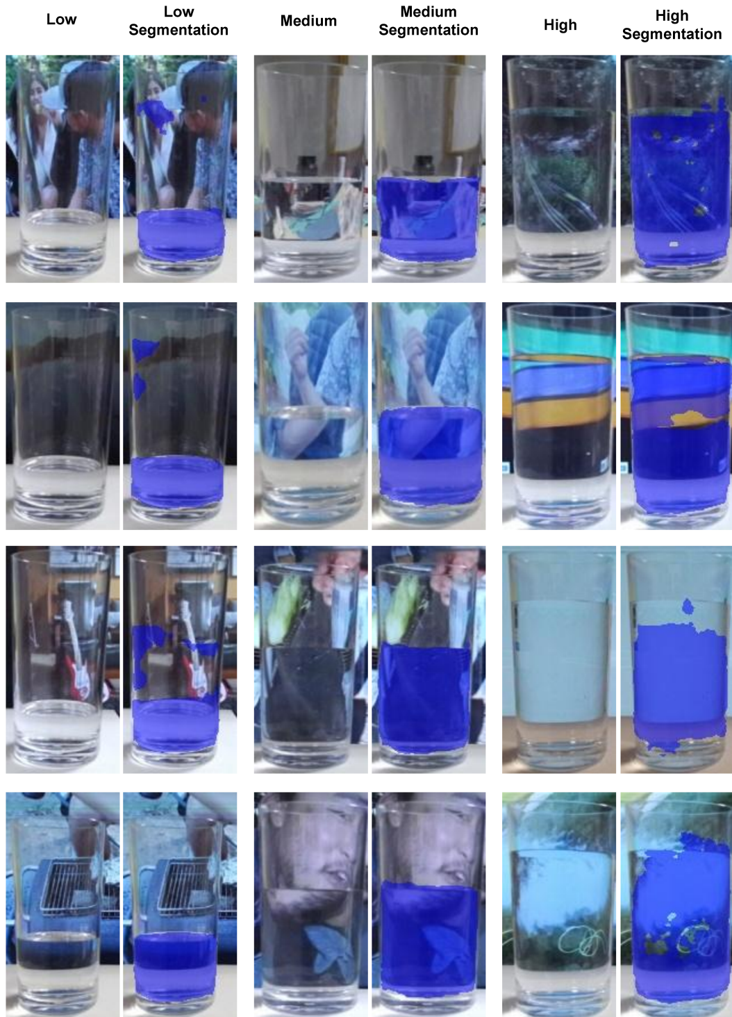
Fig. 9: We show evaluations for transparent liquid segmentation when liquid is placed in front of various backgrounds. We show segmentation masks (blue) for short, medium and tall test cases based on the quantity of liquid placed in the container.
