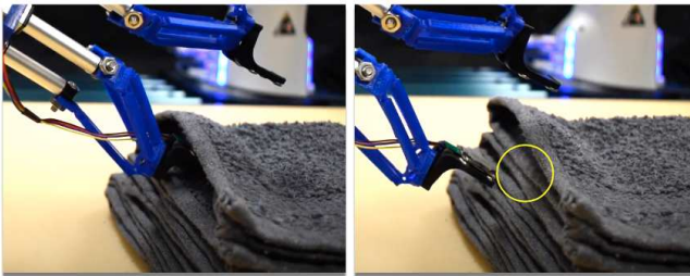
Fig. 7: A qualitative example of how the task is challenging, particularly with grasping two layers. Because of the horizontal motion of the gripper, layers of cloth can be pushed apart (left), creating air pockets between the top and second layer after the action has finished (right). This gap makes it easier to grasp the top layer but harder to grasp the top two layers, due to a smaller gap between the second and third layers (see overlaid yellow circle).
