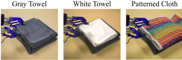
Fig. 6: The cloths we use for experiments. We use the gray towel (left) for training, and test on all 3 cloths for evaluation. The white towel and patterned cloth test generalizing to novel cloths. The cloths have thicknesses between 3-5 mm and variation in surface texture and stiffness.
