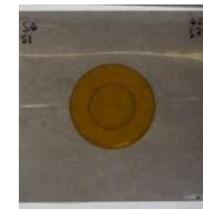
Fig. 1 Kapton® tape laser cut in the shape of a circle placed on top of a PVDF and ITO sample. The inside circle has PET and Kapton® tape whereas the outer circle is tape adhered to the ITO layer
