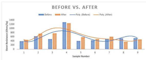
Fig. 2 Before and after measurement results for each sample. Polynomial fit lines of six degrees are shown for both the before and after results
