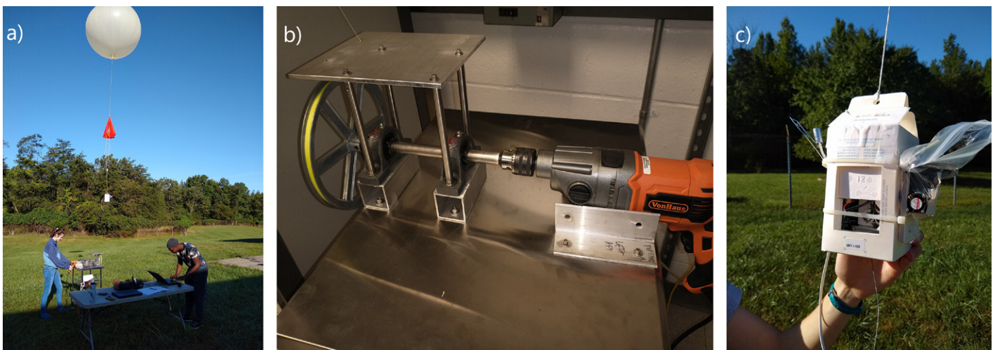
Fig. 2. (a) Early morning on 30 Aug 2019 during the tethersonde experiment with students Sara Harbison and Kofi Boateng. (b) Close-up of the tethersonde device constructed for this experiment. (c) Close-up of the iMet radiosonde with a Duke University LCS device partially enclosed in a plastic bag.
