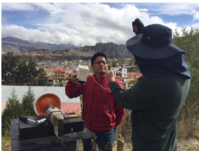
Fig. 1. Home-built tethersonde being tested by members of the LFA from the UMSA campus in La Paz on 23 Jun 2018.
