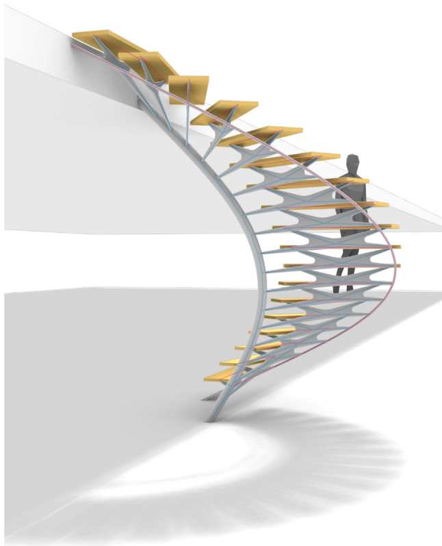
Fig. 15. Architectural interpretation of the constrained form diagram \bar{F} of a spiral staircase generated with the extended CEM framework.
