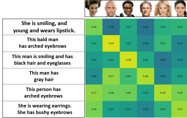
FIGURE 4. The encoder model similarity matrix, showing confident matches along the diagonal that indicate the similarity between the images of interest and their appropriate text descriptions. The prediction outputs along the diagonal is enhanced by the inclusion of the vision section of the pre-trained CLIP model.
