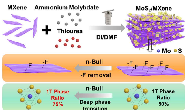
Figure 1. Schematic illustration of n -Buli treatment for MoS 2 /MXene nanohybrid structures.
