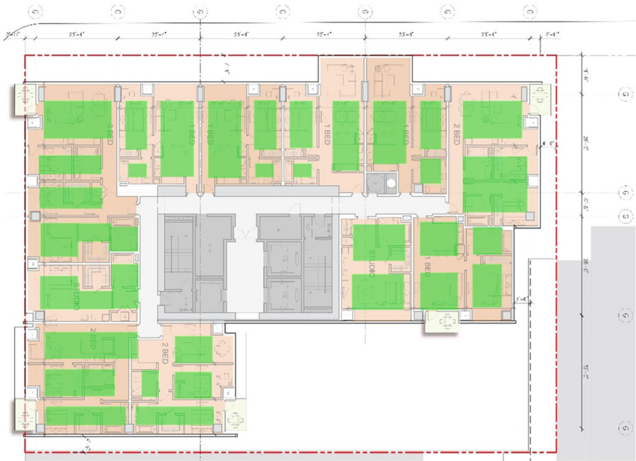
Fig. 16.1 Typical floor plan of high-rise residential complex – green geometries represent wood inlays within slab
