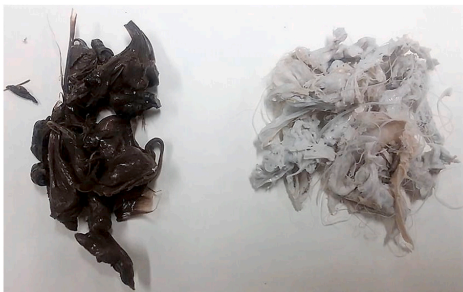
Fig. 10. Batch-to-batch variations in discoloration upon twin-screw melt-mixing of alpha-alumina filler particles into FEP resin under seemingly identical conditions ( 320^\circ\text{C} , 12 rpm, 8 min). Only more heavily discolored composite to the left results in extreme wear resistance of Fig. 3.
