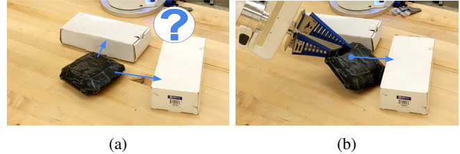
Fig. 1: Slide-to-Wall task with fixture ambiguity. (a) There are two visually identical candidate fixtures in the workspace (i.e., white boxes), only one of which is heavy enough to leverage. (b) The target object can only be grasped if the robot pushes it against the correct fixture (i.e., the box on the right).
