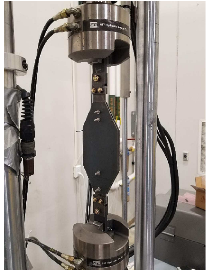
Fig. 7. Setup used for experimental axial testing of BRB analog. BRB analog is being held in loading frame with hydraulic grips. LVDT is not attached.
