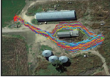
Fig. 3: Trajectory of Large number of UAVs with time while avoiding multiple obstacles
