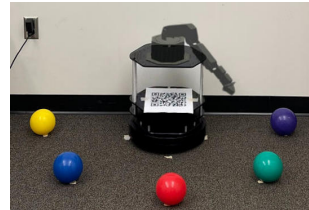
(c) Physical Robot with a virtual (AR) arm pointing to a physical referent (V→P)
