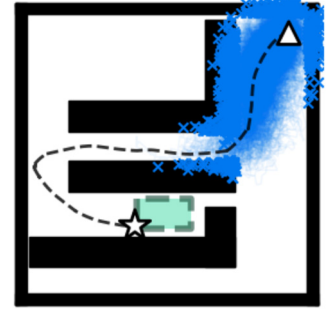
Fig. 9. Results of 1000 independent Monte-Carlo trials using zero-mean noises w_t, v_t sampled from multivariate Laplacian distribution with covariance matrices \Sigma_w = \Sigma_v = 10^{-2}I_n are shown here. With noises being strong, success rate falls to 0%. The white triangle, star and green rectangle denote the starting position, goal position and the goal region respectively.
