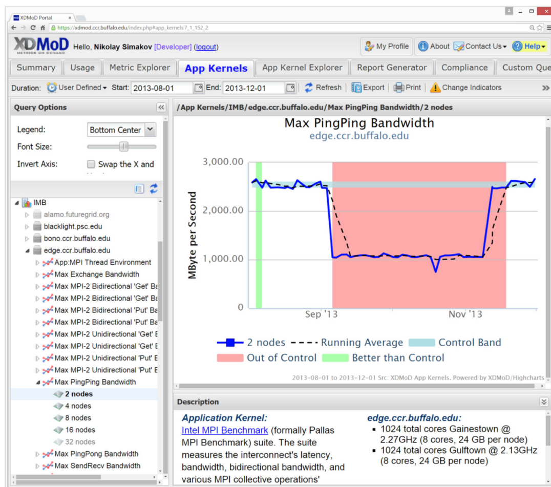
Figure 3. Application kernel process control. The time history for the network benchmarking application kernel, Intel message-passing interface (MPI) benchmarks (IMB), demonstrates an underperforming region. The solid blue line is the data, the dashed black line is a five-point average, and the blue shading indicates the control zone range. The red zones indicate that the process is out of control in an unfavorable sense, while the green zones indicate superior performance compared to the in-control performance.
