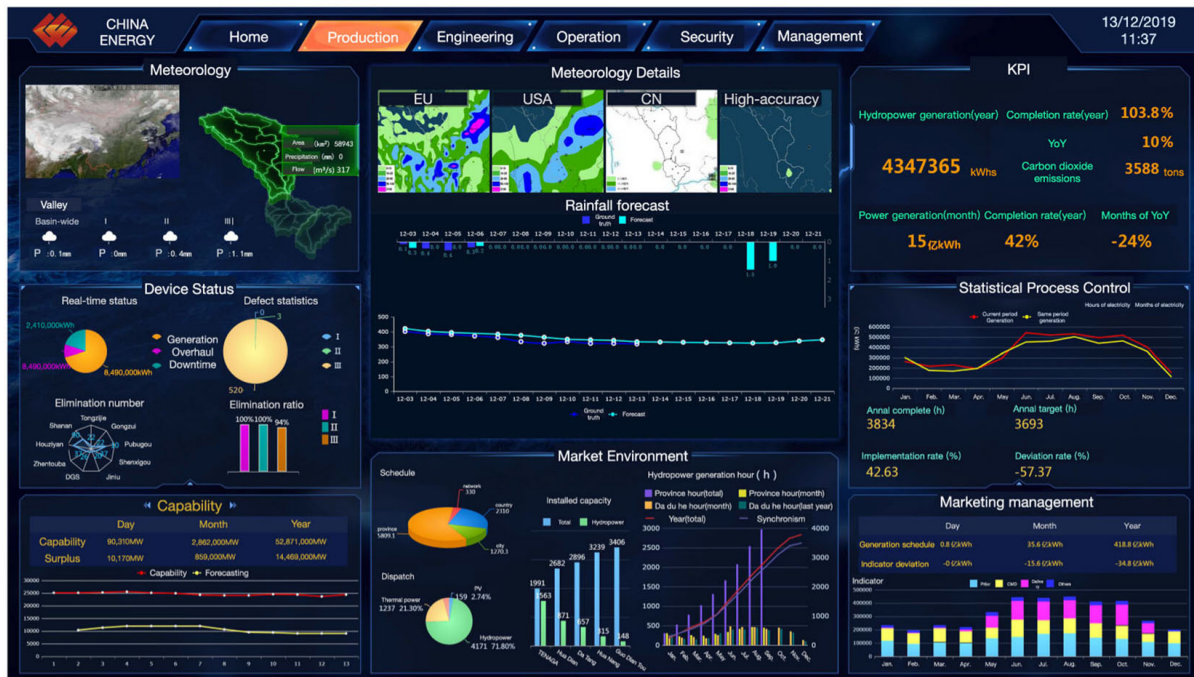
FIGURE 10 User interface of the deployment platform. There exists our hydropower demand prediction results and various IIoT sensors monitoring data for industrial operations and decisions making. IIoT, Industrial Internet of Things; KPI, key performance indicator [Color figure can be viewed at wileyonlinelibrary.com ]
