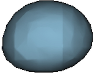
Fig. 23. Simulated shape of a 3 mm falling raindrop at low resolution D/\Delta x = 8 .
