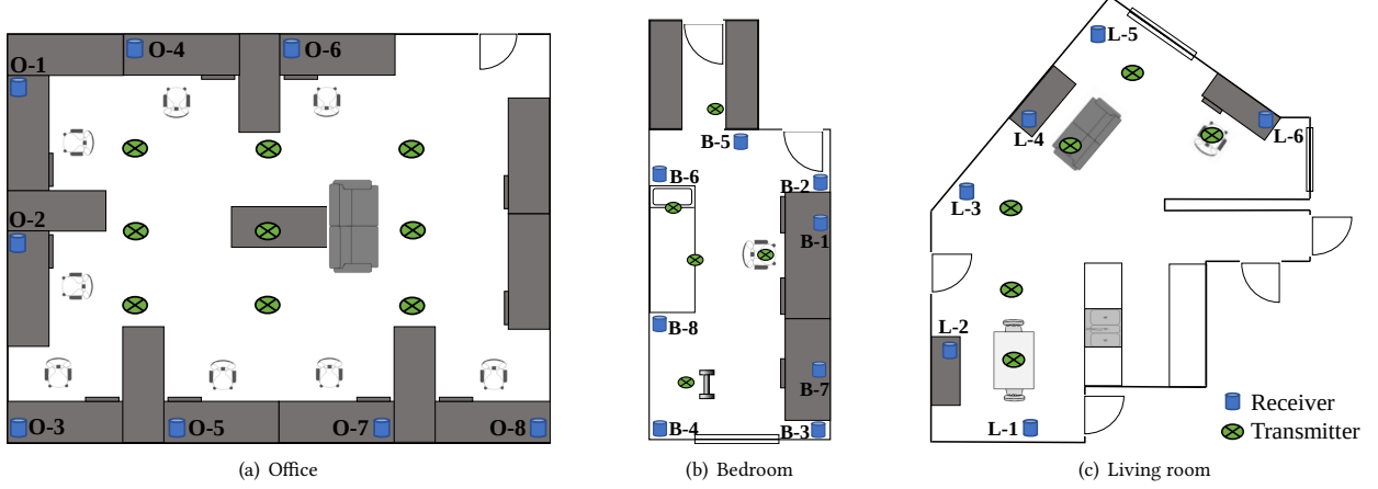
Figure 1: Deployment plan of (a) office, (b) bedroom and (c) living room. Blue cylinders denote the candidate locations of the receiver and green crossed circles denote the locations of the transmitter. The sensing quality of each blue location is determined using all the data transmitted from each green transmitting location.
