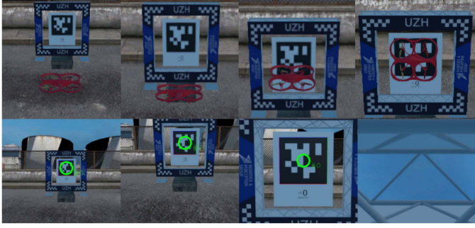
Fig. 8. Virtual perching in simulation. The top four images are the view of the quadrotor in the simulated environment. The bottom four images display the view from the camera with tag detection. The green circle denotes the target detection.
