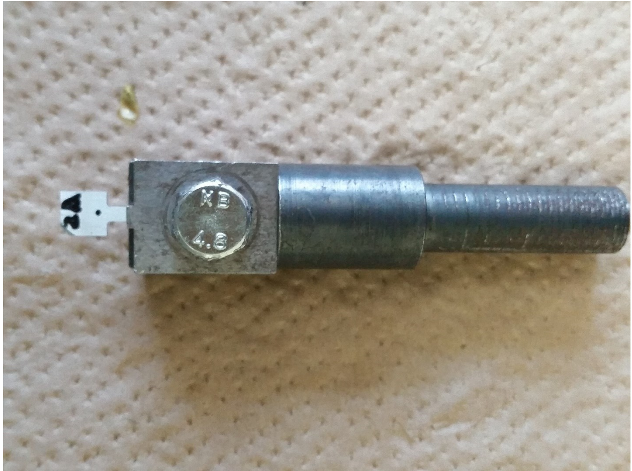
Tensile sample holder with sample in the holder.
