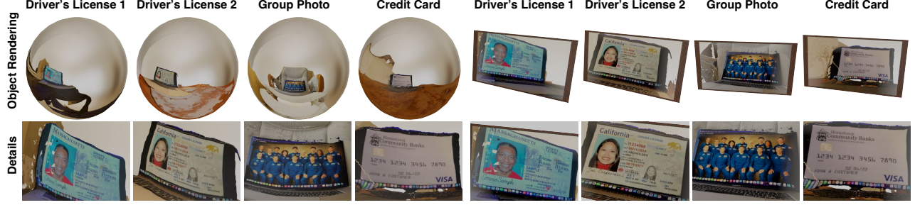
Figure 4: The visual effectiveness of our attack on reflection-based privacy. Row one shows the reflection rendering of two virtual objects; row two zooms in on the four types of sensitive information leakage.
