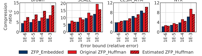
Fig. 22: Compression ratio of ZFP_Embedded , ZFP_Huffman .
