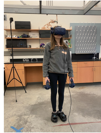
Fig. 3. The equipment used in both experiments. As seen, the Vive Pro HMD was worn, along with the handheld controllers and two Vive Trackers placed on the feet.
