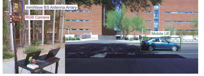
Fig. 3. System setup of the DeepSense 6G Scenario 8. The mmWave BS antenna arrays operating at 60GHz receives the signal transmitted by the moving UE. A Camera is placed under the BS to obtain sensing information.
