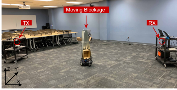
Fig. 3: Data collection setup for indoor scenario, where a blockage moves along a trajectory between the transmitter (TX) and the receiver(RX).
