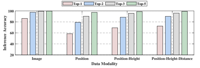
Fig. 4. This figure plots the top-k accuracies ( k \in (1, 2, 3, 5) ) for the proposed sensing-aided beam prediction solution. It is observed the vision-aided beam prediction solution outperforms the other approaches.
