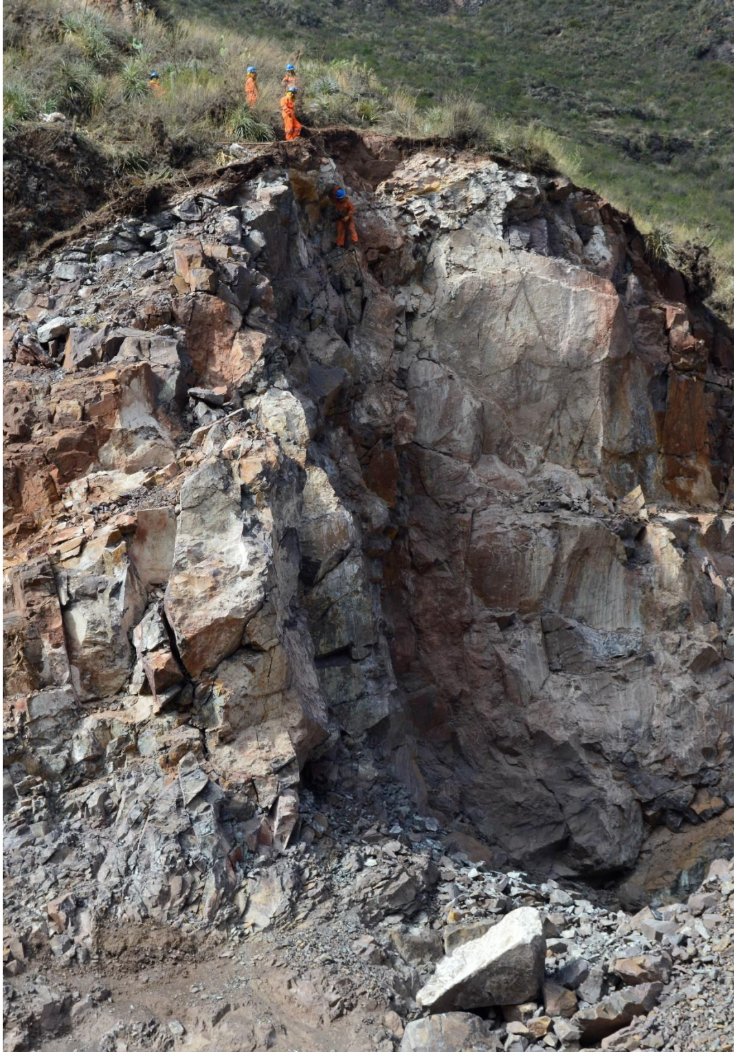
Figure 6. Modern workers quarry material from a subterranean limestone deposit near Coya. The workers first used explosives to “open” the deposit before subsequently extracting larger pieces of material by fracturing the top of the deposit with mechanical tools. The resulting morphology closely resembles pre-Hispanic quarries.
