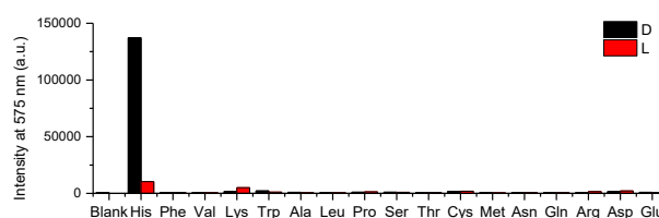
Figure 4. Fluorescence intensity at \lambda_2 = 575 nm for ( S )- 3 (0.5 mM) + Zn(OAc) 2 (2.0 equiv) with 17 pairs of amino acid enantiomers (10 equiv) ( \lambda_{\text{exc}} = 505 nm, slit: 5/5 nm. Solvent: DMF/H 2 O = 1/1 with 12.5 mM pH = 6.4 phosphate buffer).
