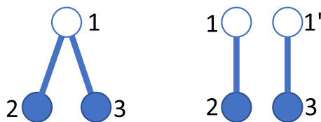
FIG. 3. Example of additional graphs that contribute to virial coefficients for flexible molecules. In deriving the density series for B_3 , the singly connected graph on the left and the disconnected graph on the right are differenced. For rigid molecules, this difference is zero. For flexible molecules, the interactions of molecule 2 with molecule 1 affects the latter's conformations, which, in turn, affects its overall interactions with molecule 3 (and vice versa). In the graph on the right, the interactions of 2 and 3 with 1 and 1' (respectively) are independent. The net result is that the difference is nonzero. A solid "field" point represents an integral over a molecule's position and conformation, while an open "root" point represents an integral over only conformation. Bonds represent Mayer f -function. 5
