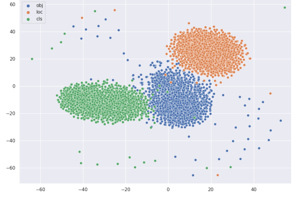
Fig. 2: Visualization of adversarial examples generated from different task losses using t-SNE. Different colors encode the task losses used for generating adversarial examples (blue: objectness, orange: localization, green: classification loss). This is a typical example from the KITTI dataset for autonomous driving.
