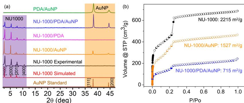
**Figure 2.** (a) PXRD profiles of NU-1000, AuNP, NU-1000/AuNP, NU-1000/PDA, NU-1000/PDA/AuNP, and PDA/AuNP. (b)  $\text{N}_2$  sorption isotherms (77 K) of pristine NU-1000 (black), NU-1000/AuNP (orange), and NU-1000/PDA/AuNP (blue), adsorption: closed circles, desorption: open circles.
