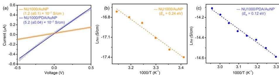
**Figure 4.** (a) Representative  $I$ - $V$  plots of NU-1000/AuNP (orange) and NU-1000/PDA/AuNP (blue). Arrhenius plots of temperature-dependent conductivity of (b) NU-1000/AuNP (orange) and (c) NU-1000/PDA/AuNP (blue) revealing their respective activation energies.
