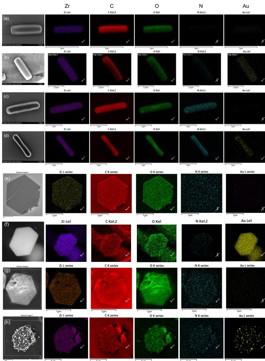
**Figure 3.** (a–d) The SEM images (left) and color-coded STEM-EDX elemental mapping (right) of (a) pristine NU-1000, (b) NU-1000/AuNP, (c) NU-1000/PDA, and (d) NU-1000/PDA/AuNP. (e–h) Cross-sectional SEM images (left) and color-coded STEM-EDX elemental mapping (right) of (e) pristine NU-1000, (f) NU-1000/AuNP, (g) NU-1000/PDA, and (h) NU-1000/PDA/AuNP.
