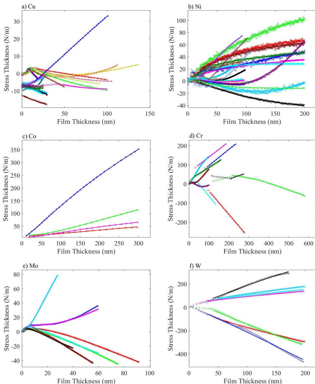
**Fig. 2.** Data (symbols) and model fit (line) for (a) Cu, (b) Ni, (c) Co, (d) Cr, (e) Mo and (f) W. The processing conditions and source of the data corresponding to each color in the figure can be found in the corresponding tables in the supplemental material.
