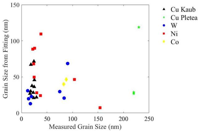
Fig. 4. Grain size from fitting vs measured grain size. The calculation from the fitting parameters is done at the same thickness as the measurement.
