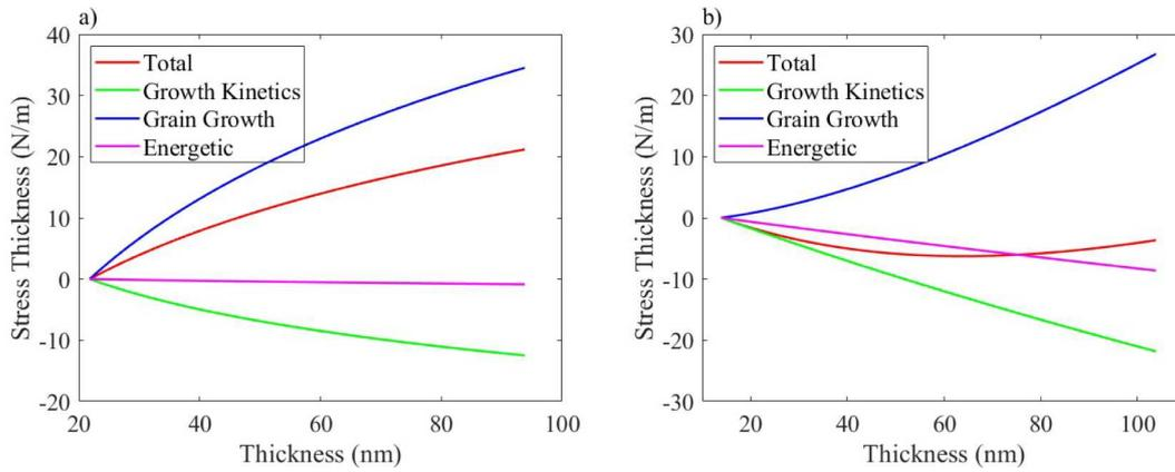
**Fig. 1.** Plots showing the different components of the stress model, as indicated in the legend, for different processing conditions for sputtered Ni from Lumbeck [24]. (a) 1.07 Pa 300 K 0.016 nm/s, (b) 0.27 Pa 300 K 0.034 nm/s.
