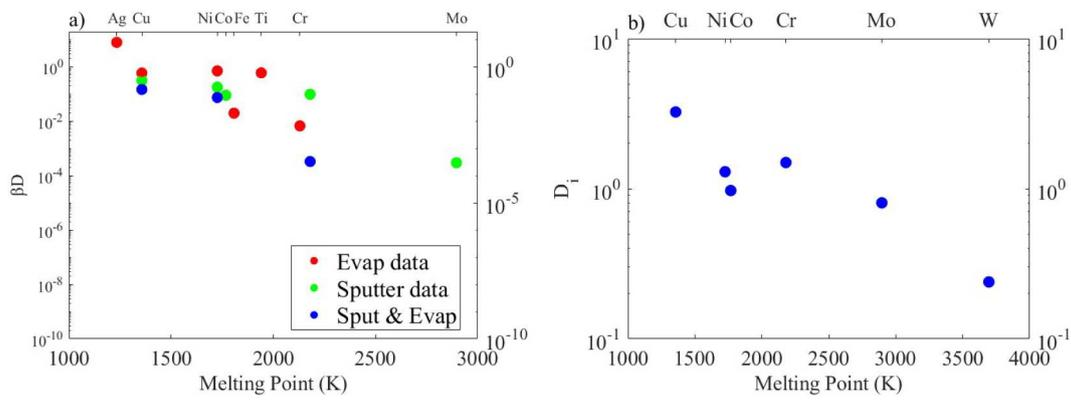
Fig. 3. Fitting parameters for diffusional kinetics determined at room temperature vs melting point of material. (a)  $\beta D$ , (b)  $D_i$ .
