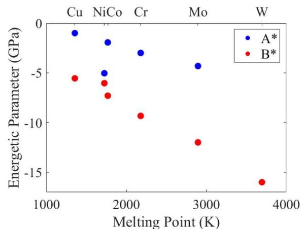
Fig. 5. Fitting parameters  $A^*$  and  $B^*$  for energetic terms vs the melting point of the material.
