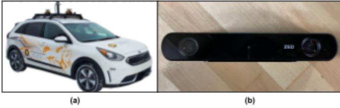
Figure 2. (a) Kia Niro Instrumented Research Vehicle, (b) ZED 2 stereo camera.
