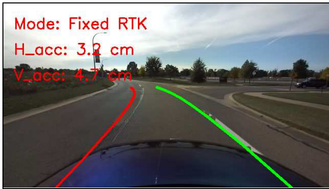
Figure 18. Campus Drive camera frame from a curved road segment with high-definition map lane line data overlaid on artificially occluded lane lines. Deviation from true lane lines occurs in this curved road segment due to the insufficient sampling rate of the GNSS heading sensor.
