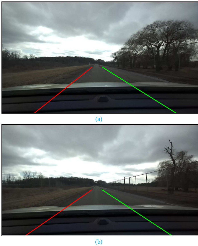
Figure 15. Two examples of Eaton Proving Grounds camera frames from straight road segments with high-definition map lane line data overlaid on artificially occluded lane lines. These show well-aligned lane lines.
