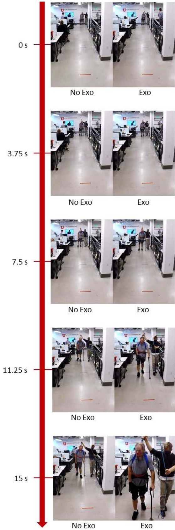
Fig. 3. Ten-meter walking test. Still frames from the supplementary videos show the visual difference between using the exoskeleton and not using the exoskeleton.
