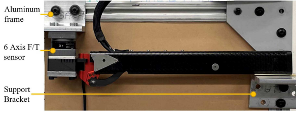
Fig. 7. Bench set up for step response. The exoskeleton crank was connected to a load cell, grounded to a rigid frame. The carbon fiber frame was braced against a rigid bracket. Free body diagrams of each system (red and blue) are shown.
