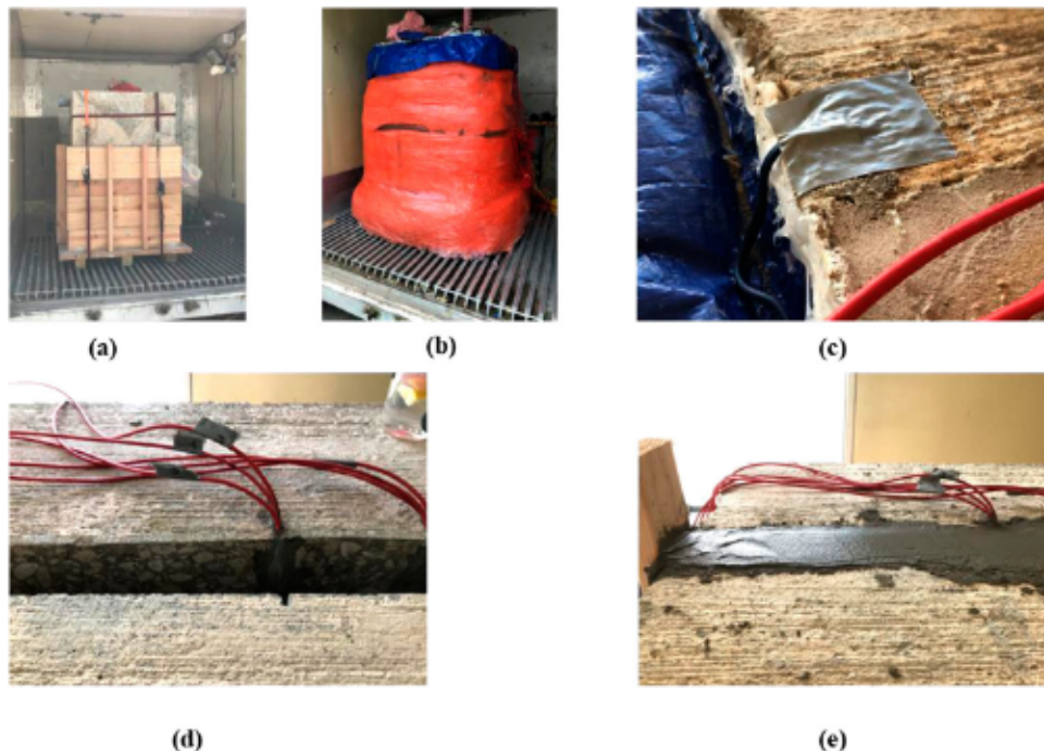
Figure 3. (a): Complete system installed in the freezer box (b): Insulation wrapping (c): Installation of edge surface thermocouple (d): Gap between the slabs prior to filling (e): Gap after filling.
