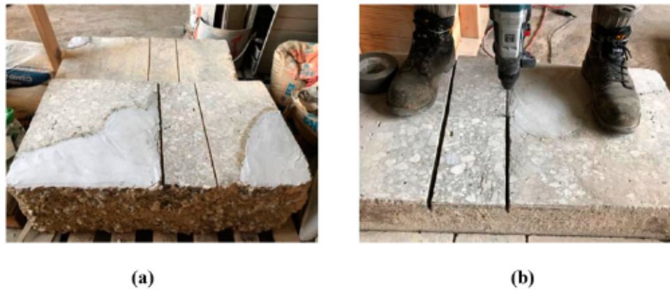
Figure 2. (a): Slab after repair (b): Drilling holes for sensor heads.
