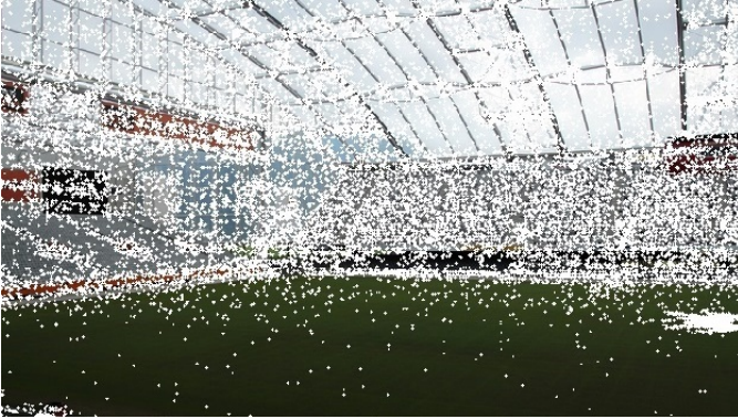
Fig. 7. Example of accurate localization results from ESAC on the RS dataset. We render the sparse point cloud from COLMAP over the input images using the pose estimate. An accurate localization results in good alignment of the keypoints (white) with their corresponding structures in the image.
