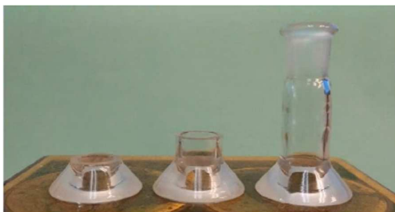
Fig. 7. Low-, medium- and high-top Franz diffusion cell caps available in our laboratories (GBK, LX). The caps used to calibrate the UB/UC model were similar to the leftmost picture. The caps used in the CE study (Hewitt et al., 2019) had approximately the same height as the top in the middle picture, but also a different design and mounting configuration as described in the text.
