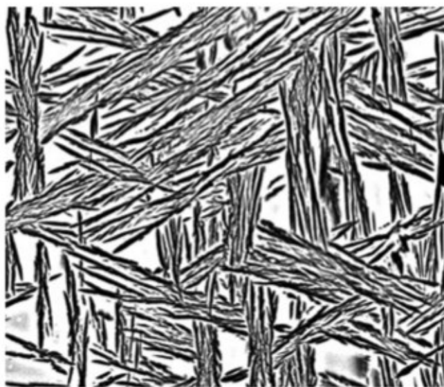
Figure 1. Microstructure of \alpha in a Ti-5.5 at %Mo alloy after aging at 700°C.
