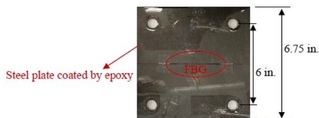
Fig. 5 An example embedded FBG sensor.
