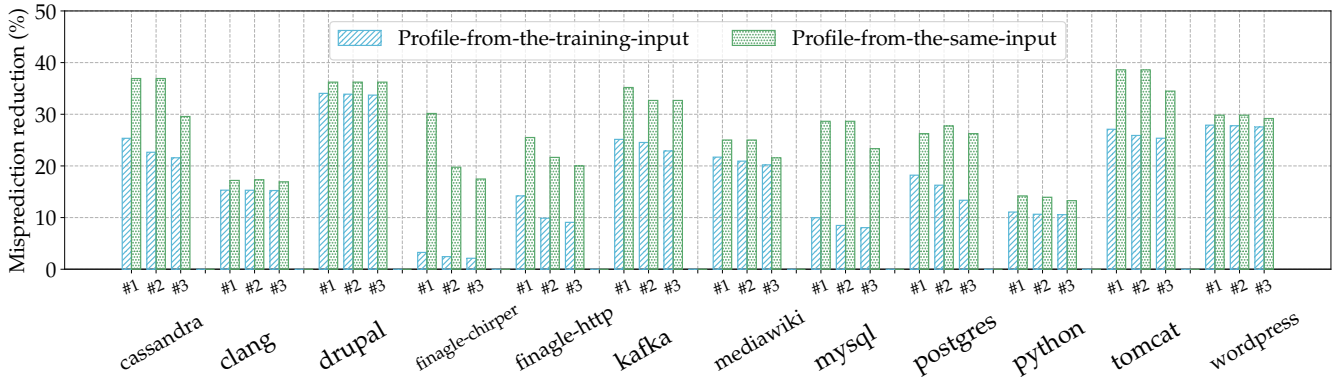
Fig. 17: Whisper ’s performance for various application inputs: On average Whisper reduces 6.6% more branch mispredictions with input-specific profiles compared to profiles from different inputs.
