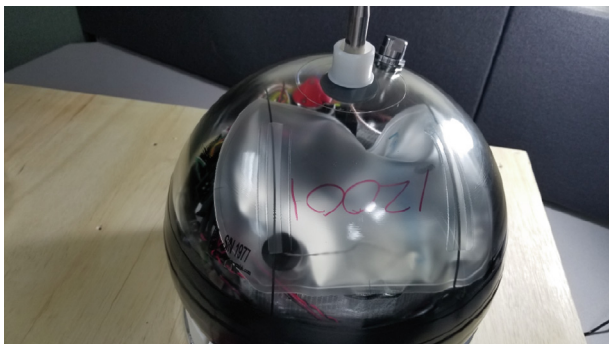
Fig. 3. Deep Argo floats, meant to measure temperature and salinity as deep as 6000 m, have been reengineered with a spherical glass casing to withstand the intense pressures at greater depths. Credit: MRV Systems (public domain).
