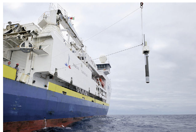
Fig. 1. Deployment of an Argo float in the Balearic Sea from the French research vessel Pourquoi Pas. Credit: Argo program (public domain).
