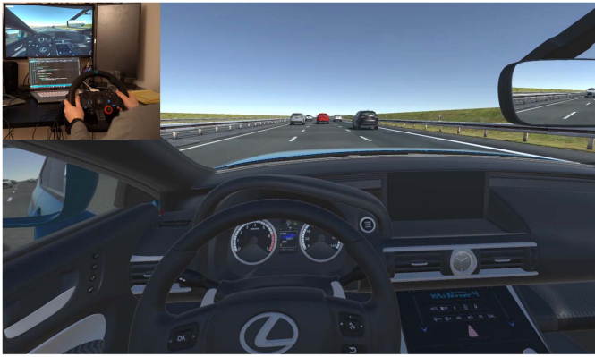
Fig. 4. Naturalistic driving in a car-following scenario with a gaming laptop, a Logitech racing wheel, and the Unity game engine.
