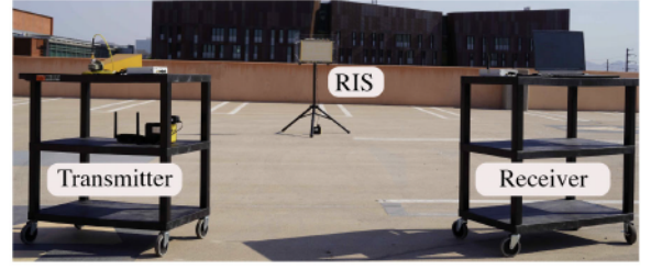
FIGURE 15. The RIS-assisted wireless communication system consists of an RIS, a transmitter (BS), and a receiver (UE). The transmitter and receiver are portable and can be placed in the far-field of the RIS surface.
